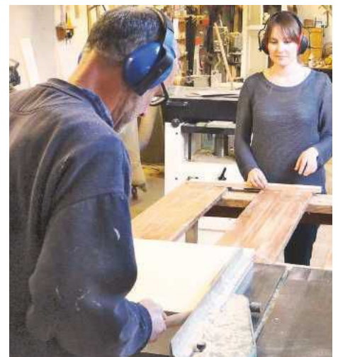
▲ Pic.5 Richard has extended his saw table so that he can rip an 8 x 4ft sheet single-handedly. Imogen is largely unnecessary here but she witnessed the very beginning of her coffee table, and loved it
